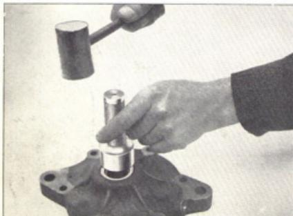
FIG. 5. Removing the roller race outer ring and the oil seal from the drive end cover.
