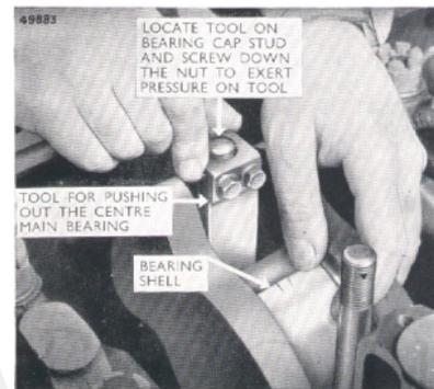
Fig. 48. Removal of main bearing shell.
