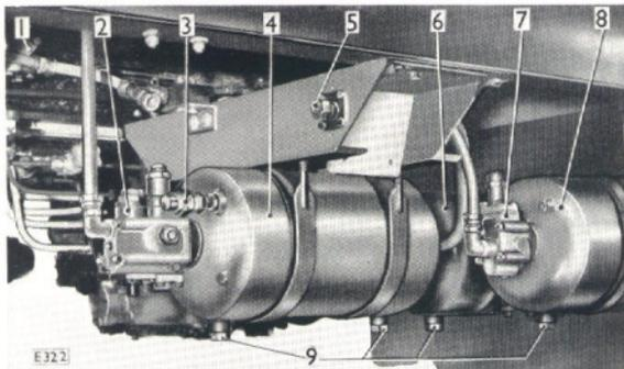
Fig. 5. Air reservoirs, unloader and diverter valves.
