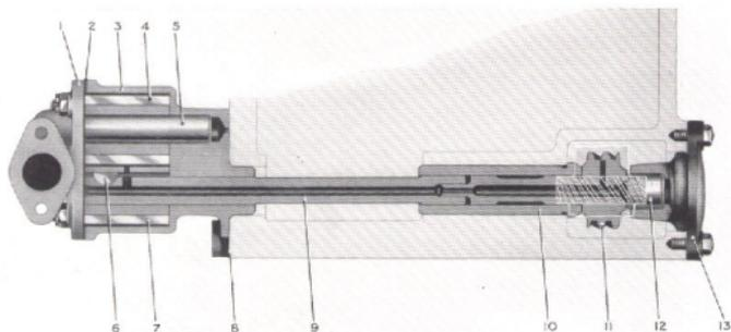
Fig. 12. Plan view of oil pump and drive.
