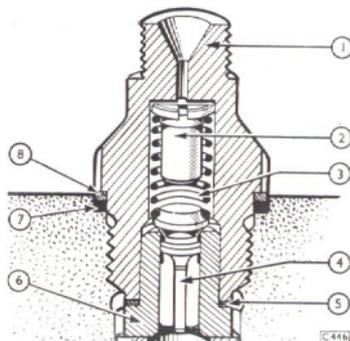
Fig. 35. Section through "N" type pump delivery valve assembly.
