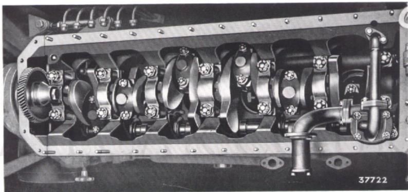
Fig. 45. Crankshaft in position.
