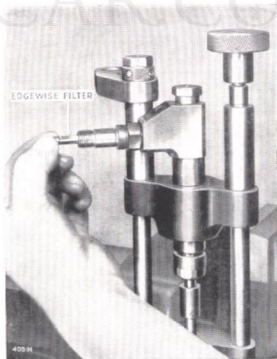
Fig. 73. Fitting the edgewise fuel filter.
