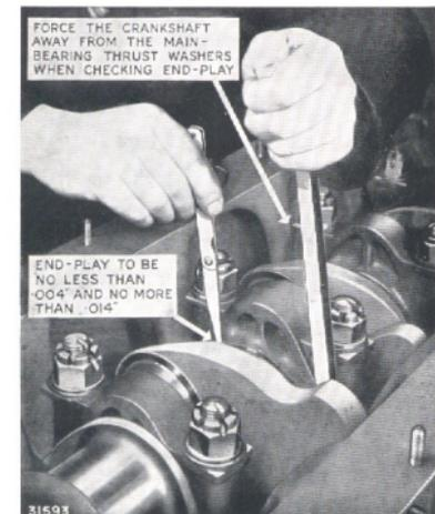
Fig. 52. Checking crankshaft end-play.
