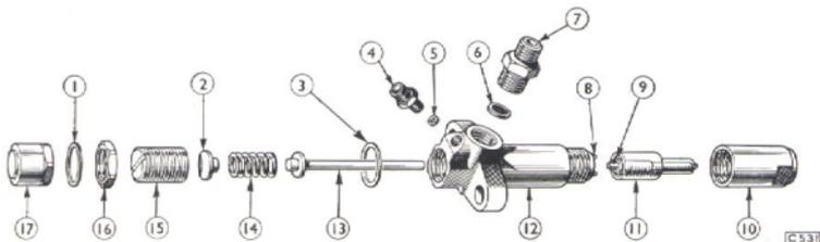
Fig. 24. Exploded view of injector.
