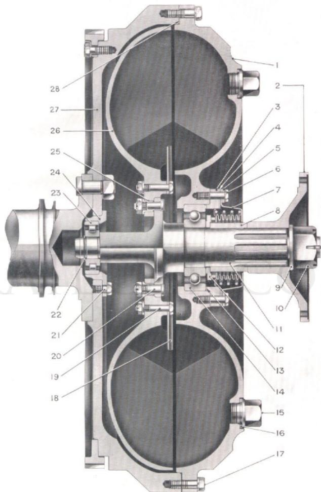
Fig. 1. Section through fluid coupling (L-type).
