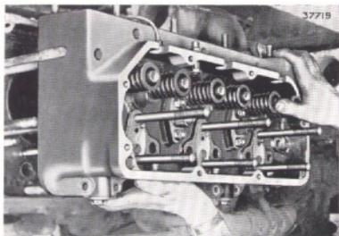
Fig. 26. Removing the cylinder heads.
