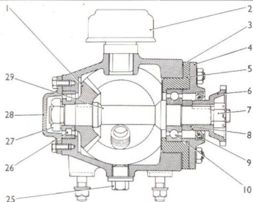
Fig. 62. Arrangement of right-angle fan drive unit.
