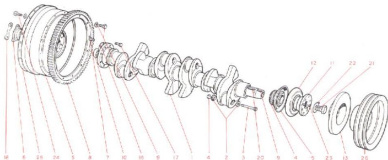
Fig. 54. Exploded view of crankshaft.
