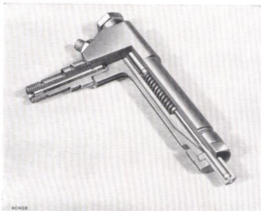
Fig. 61. An injector unit sectioned.
