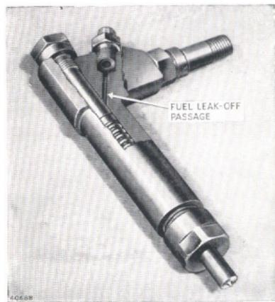
Fig. 66. Part sectioned view of injector unit.
