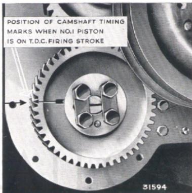
Fig. 38. Camshaft timing marks.
