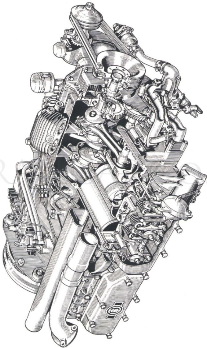
Fig. 1. Cut-away view of the (L - type) engine.
