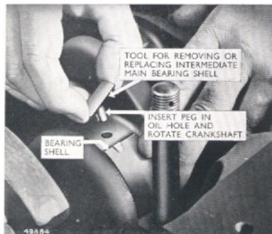
Fig. 47. Removal of intermediate bearing shell.
