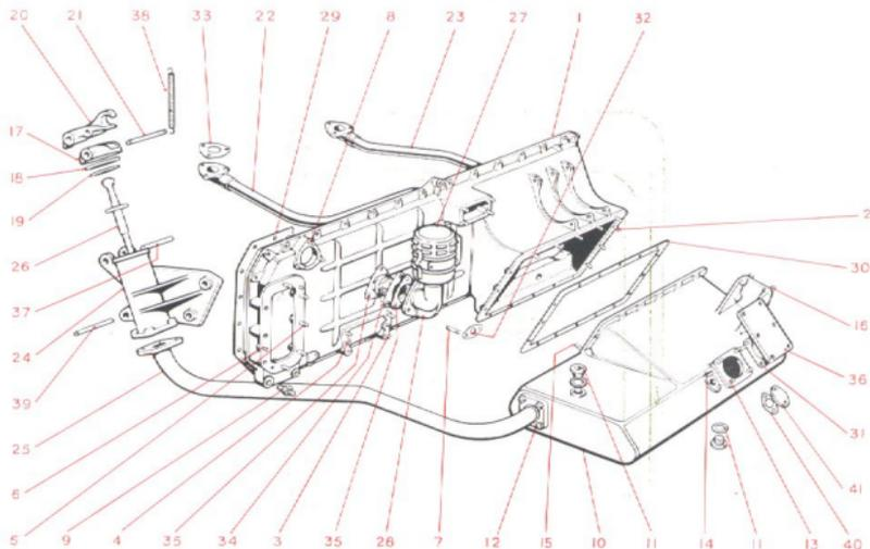
Fig. 11. Exploded view of the engine sump.
