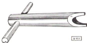
Fig. 64. Tool for starter motor armature spring nut.
