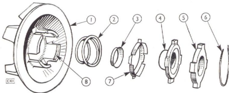
Fig. 60. Exploded view of water pump gland.
