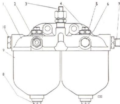
Fig. 43. Arrangement of fuel filter (C.A.V.)—twin paper element type.
