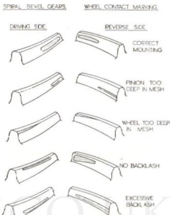
Fig. 8. Marking on teeth of spiral bevel wheel.
