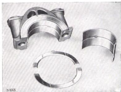
Fig. 46. Centre main bearing and thrust washers.
