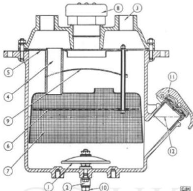
Fig. 36. Section through exhaust oil reservoir.
