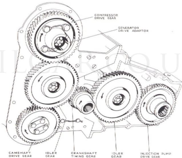
Fig. 55. The timing gears.
