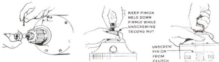
Fig. 89. Renewing starter motor pinion.
