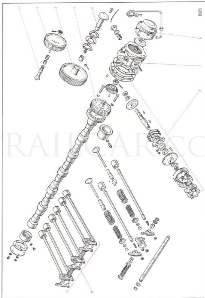
Fig. 15. Exploded view of camshaft and valve gear.
