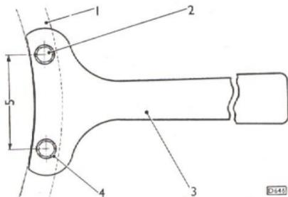
Fig. 11. Tool for turning engine crankshaft.
