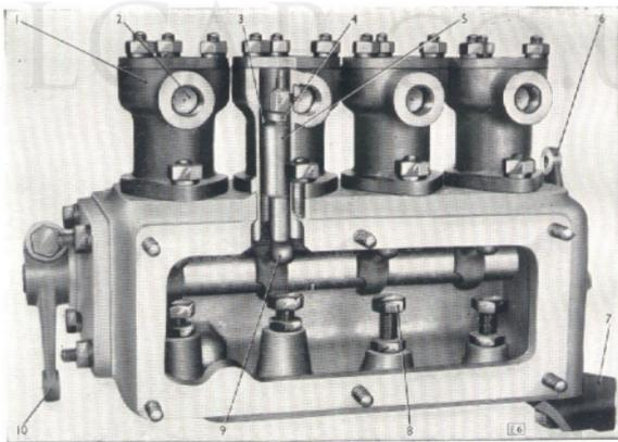
Fig. 48. Throttle motor showing cut-away view of operating piston.
