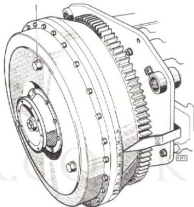
Fig. 37. Position of engine flywheel for fuel-injection pump spill cut-off point and (1) for filling or topping-up.
