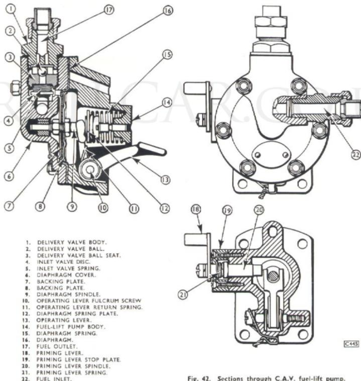
Fig. 42. Sections through C.A.V. fuel-lift pump.
