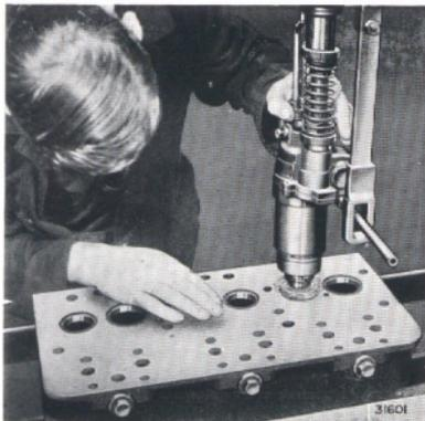
Fig. 30. Grinding valve seats.
