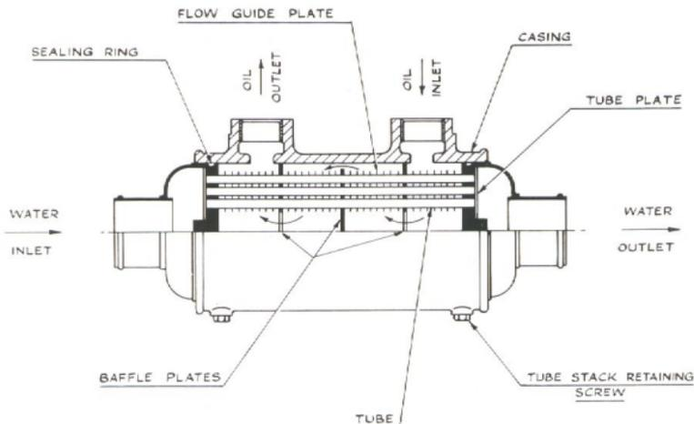
Fig. 19. Sectioned view of oil cooler.
