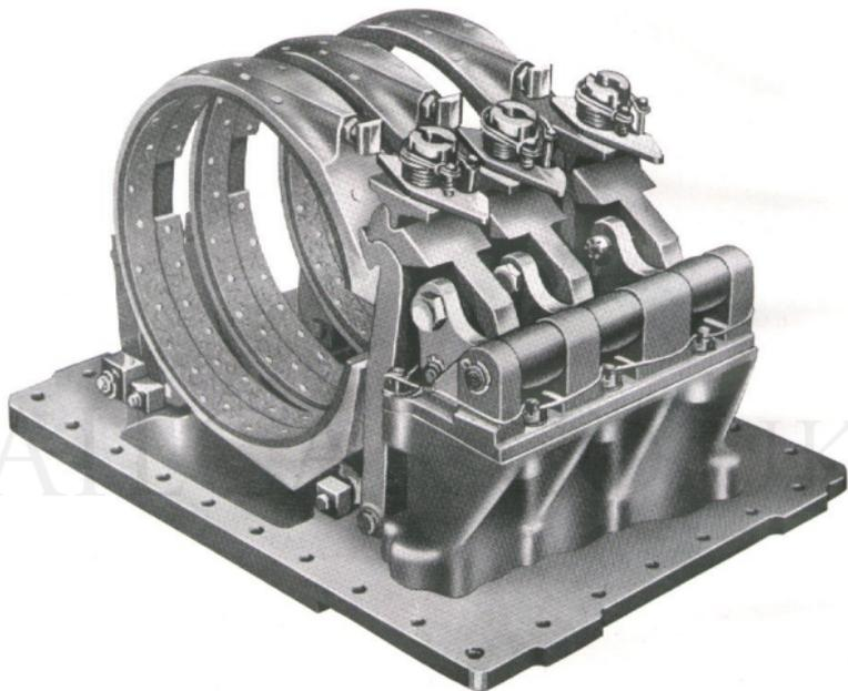
Fig. 19. The Bottom Cover and Brake Band Assembly.
