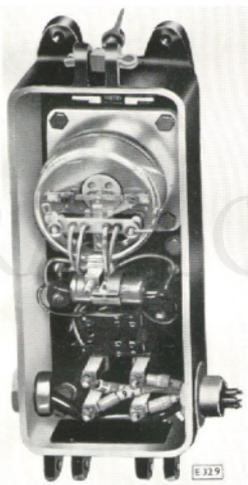
Fig. 15. Starter motor isolating relay.
