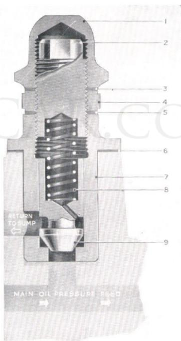
Fig. 20. Oil pressure relief valve.
