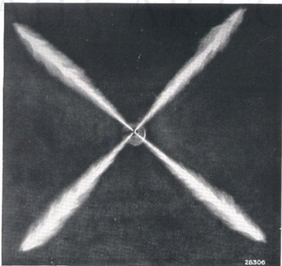
Fig. 64. Injector spray as seen by the high-speed camera.
