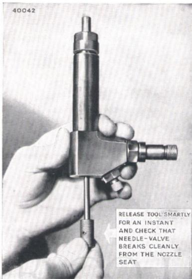
Fig. 72. The inverted test.
