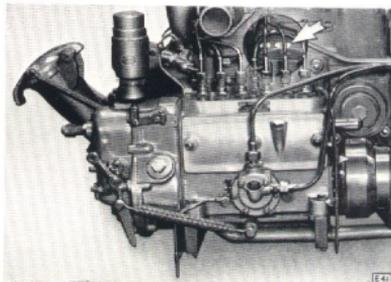
Fig. 5. Engine number stamped as indicated by arrow.
