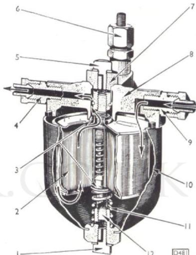
Fig. 44 Section of fuel filter (C.A.V.)—paper element type.
