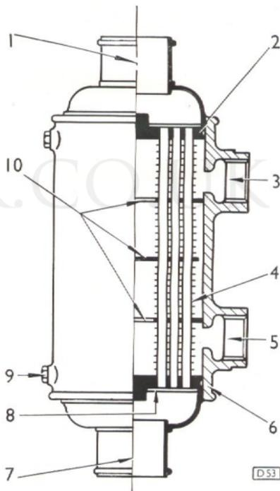
Fig. 51. Section through oil cooler.
