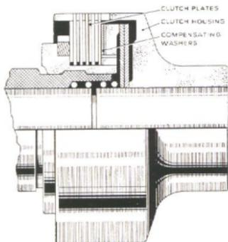
Fig. 86. Starter motor clutch.
