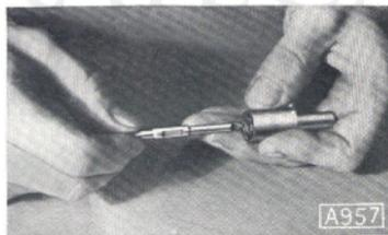
Fig. 29. Tool for cleaning nozzle seat.
