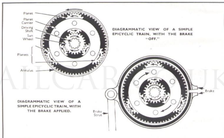
Fig. 8. Diagrammatic View of Epicyclic Gear Train.
