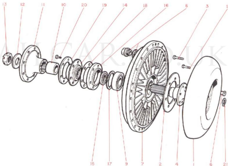
Fig. 3. Exploded view of fluid coupling (L - type).
