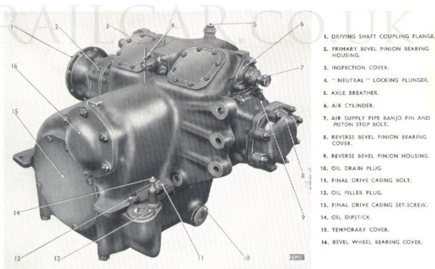
Fig. 4. Final drive unit. (The indicator switch is not shown in this illustration).
