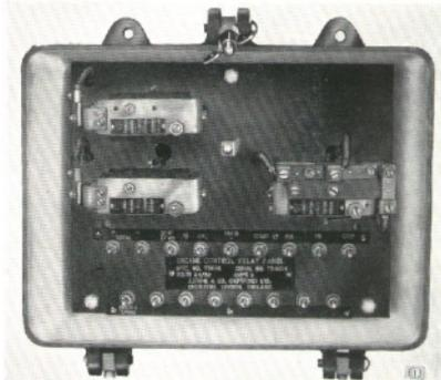
Fig. 16. Engine control relay panel.
