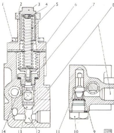
Fig. 9. Sectioned view of diverter valve.
