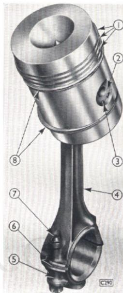
Fig. 21. Piston and connecting rod.
