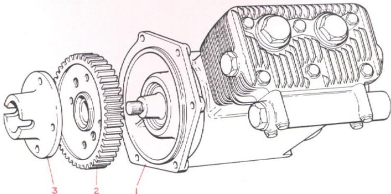
Fig. 90. The air compressor.
