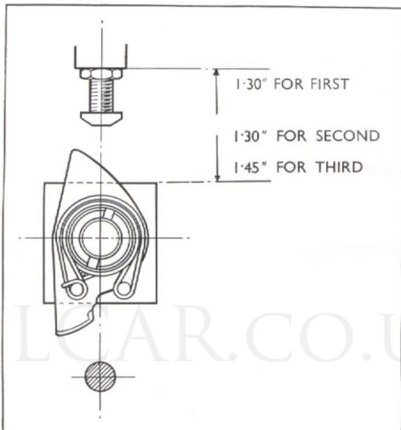
Fig. 13. Brake Setting Dimensions.
