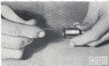
Fig. 30. Cleaning nozzle fuel passages.
