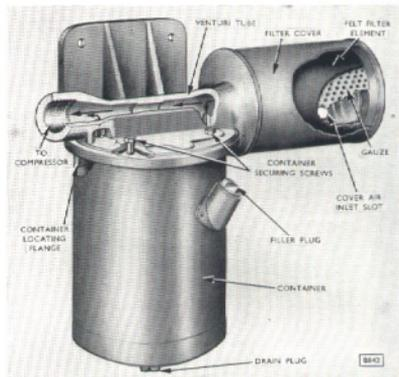
Fig. 4. Combined air filter and anti-freezer.
