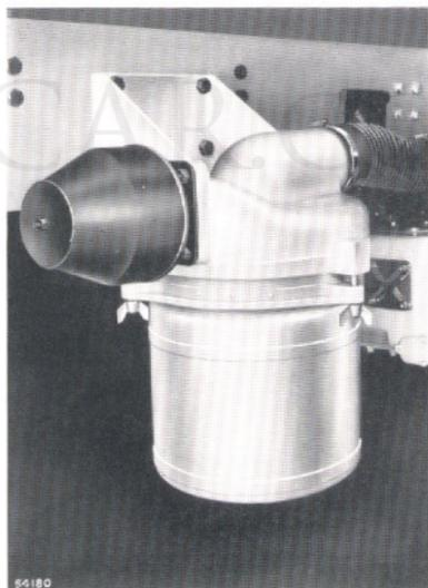
Fig. 92. The engine air cleaner.
