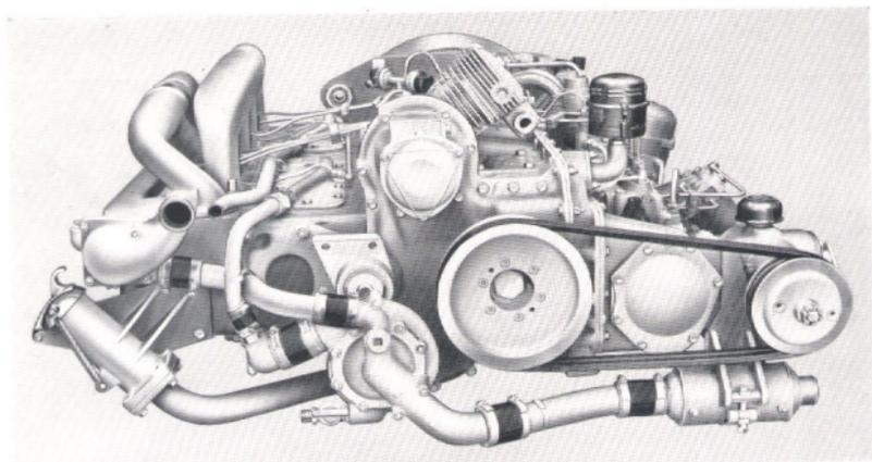
Fig. 7. Front-end view of the R.E.680 engine.
