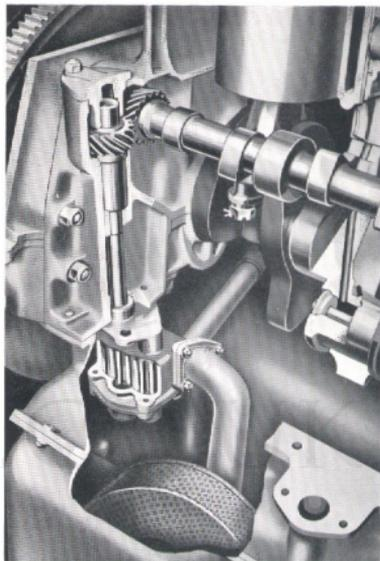
Fig. 15. Oil pump drive from camshaft (engine in stand).
