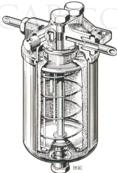
Fig. 82. Fuel filter (cloth element)
