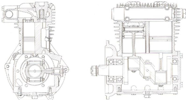
Fig. 91. Sectioned view of air compressor.
