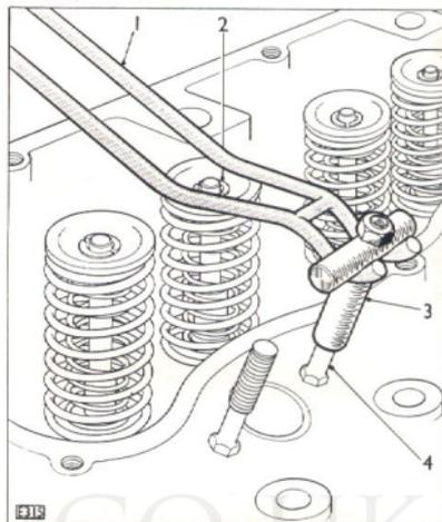
Fig. 10. Removal of valve springs.
