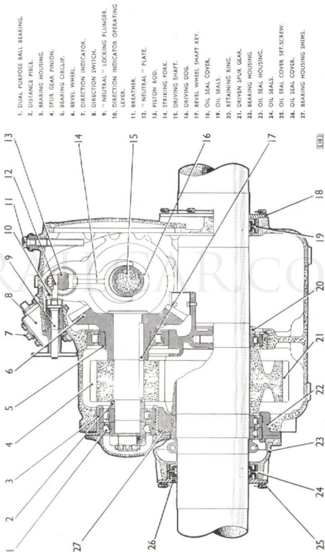
Fig. 3. Longitudinal section through bevel wheel and shaft.
