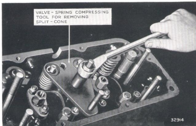
Fig. 32. Valve spring compressing tool.
