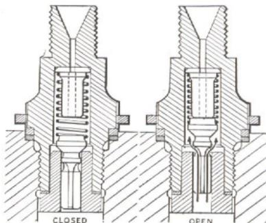
Fig. 76. Injection pump delivery valve.
