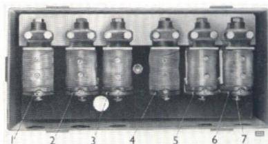
Fig. 23. Electro-pneumatic valves for engine and final drive.
