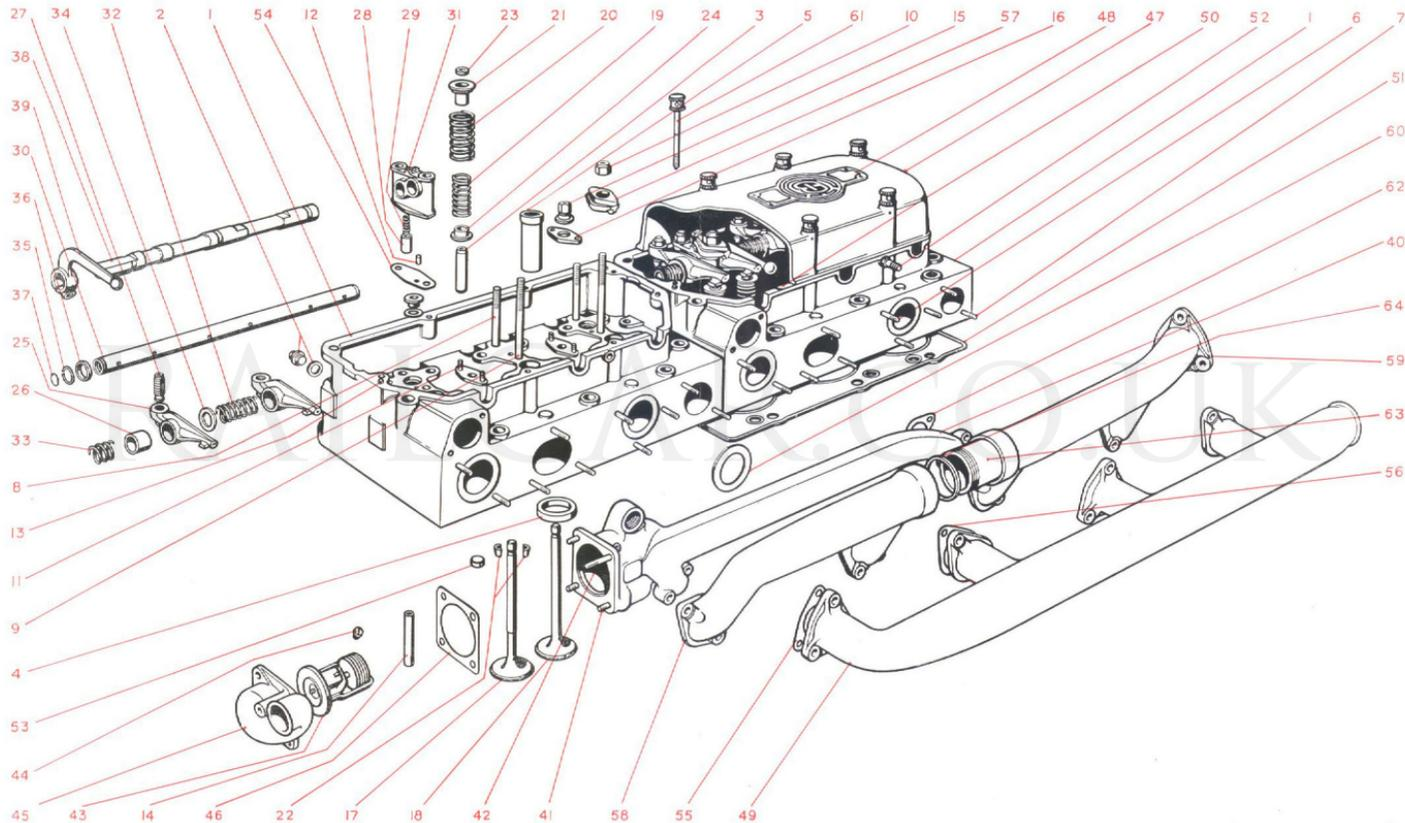
Fig. 33. Exploded view of cylinder head.
