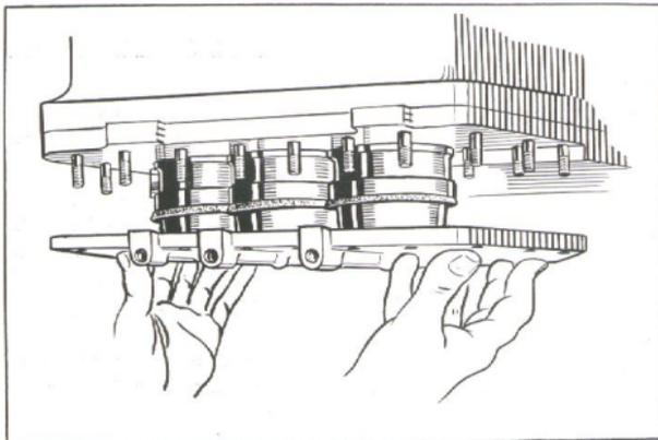
Fig. 10. Removing the Cover Plate (1st, 2nd and 3rd Speeds).
