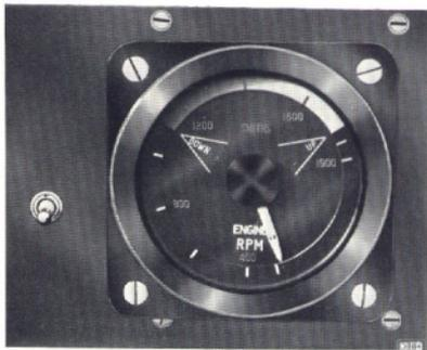
Fig. 26. Engine speed indicator and switch.
