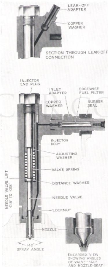
Fig. 63. The injector unit.
