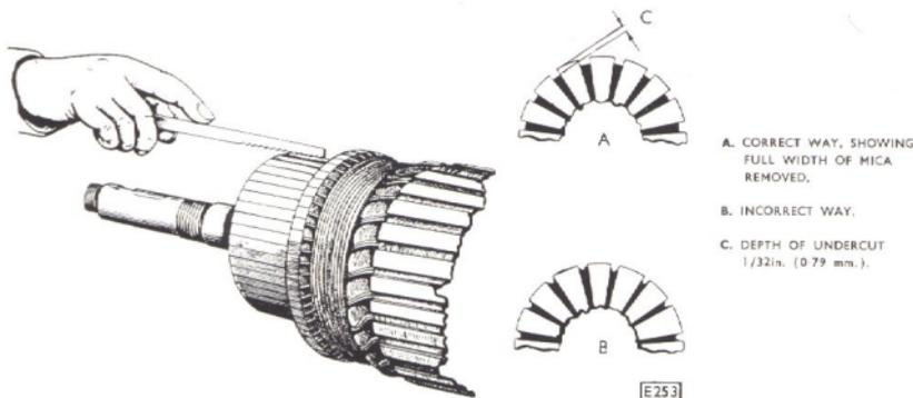
Fig. 69. Method of undercutting commutator mica.
