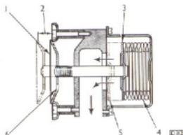
Fig. 61. Section through thermostat.
