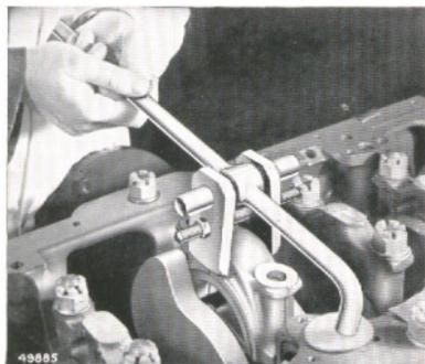
Fig. 49. Removal of bearing caps.
