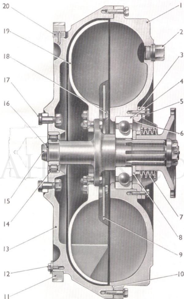
Fig. 2. Section through fluid coupling (A - type).
