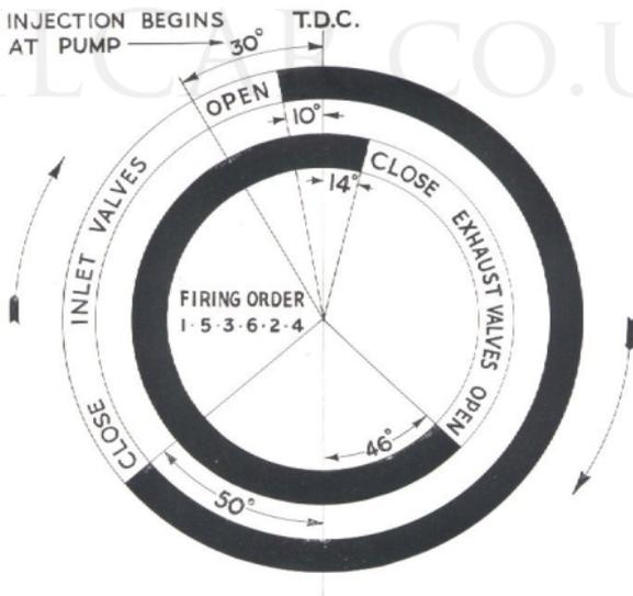
Fig. 34. Valve timing diagram.
