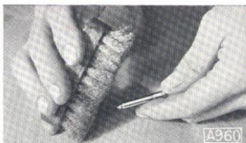
Fig. 32. Brass wire brush for cleaning nozzle valve.
