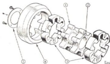
Fig. 39. Exploded view of fuel-injection pump flywheel assembly.
