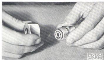
Fig. 31. Nozzle inserted in adaptor for washing.
