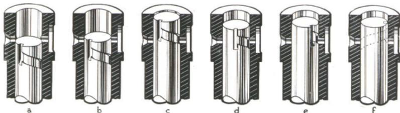
Fig. 77. The principle of fuel metering.
