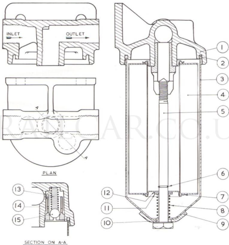
Fig. 12. Drawing of Filter.
