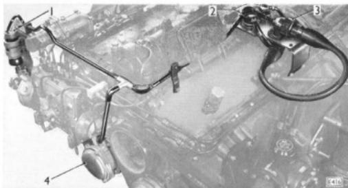
Fig. 39. Engine plug and socket, harness and conduit.
