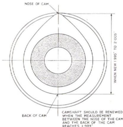
Fig. 35. Cam wear diagram.
