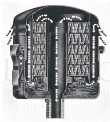
Fig. 21. Engine crankcase breather.
