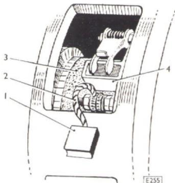
Fig. 68. Method of "bedding" starter motor brushes.
