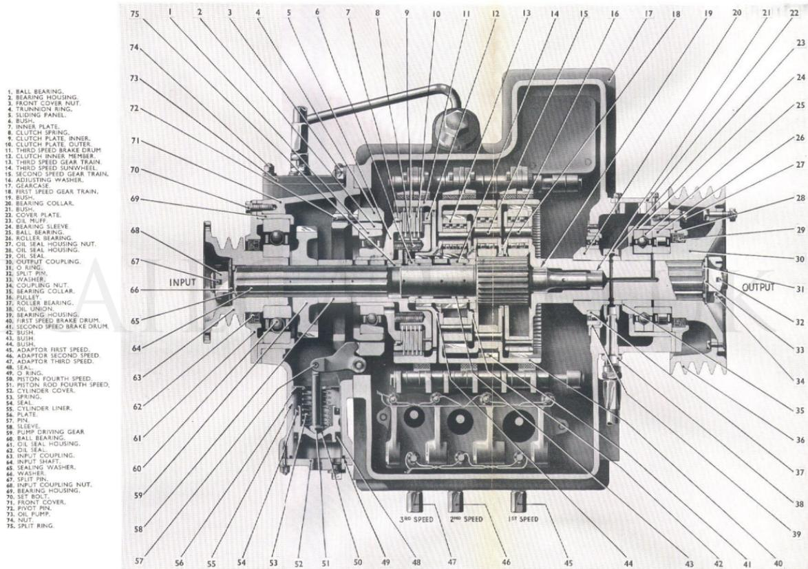
Fig. 2. Section through Gearbox.
