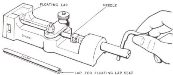
Fig. 69. Injector needle lapping jig.
