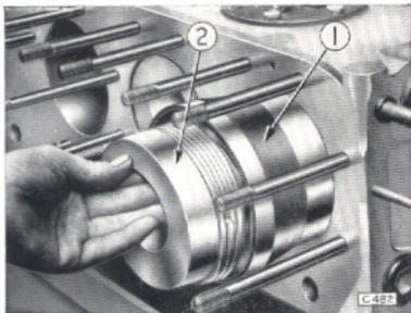
Fig. 22. Method of fitting pistons.
