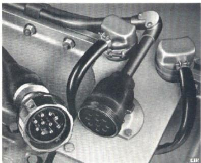
Fig. 27. Engine plug and socket.
