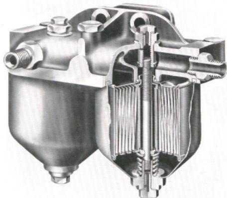
Fig. 83. Fuel filter (paper element).
