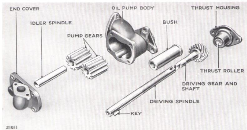
Fig. 13. Oil pump and drive dismantled.
