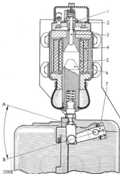
Fig. 30. Section through engine shut-down solenoid.
