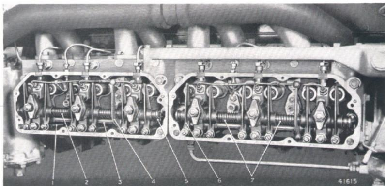
Fig. 22. Cylinder heads in position showing valve gear.
