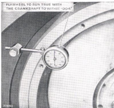
Fig. 53. Checking flywheel for running true.
