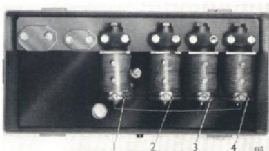
Fig. 21. Electro-pneumatic valves for gearbox.
