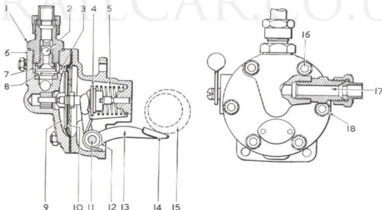
Fig. 81. Fuel feed pump.
