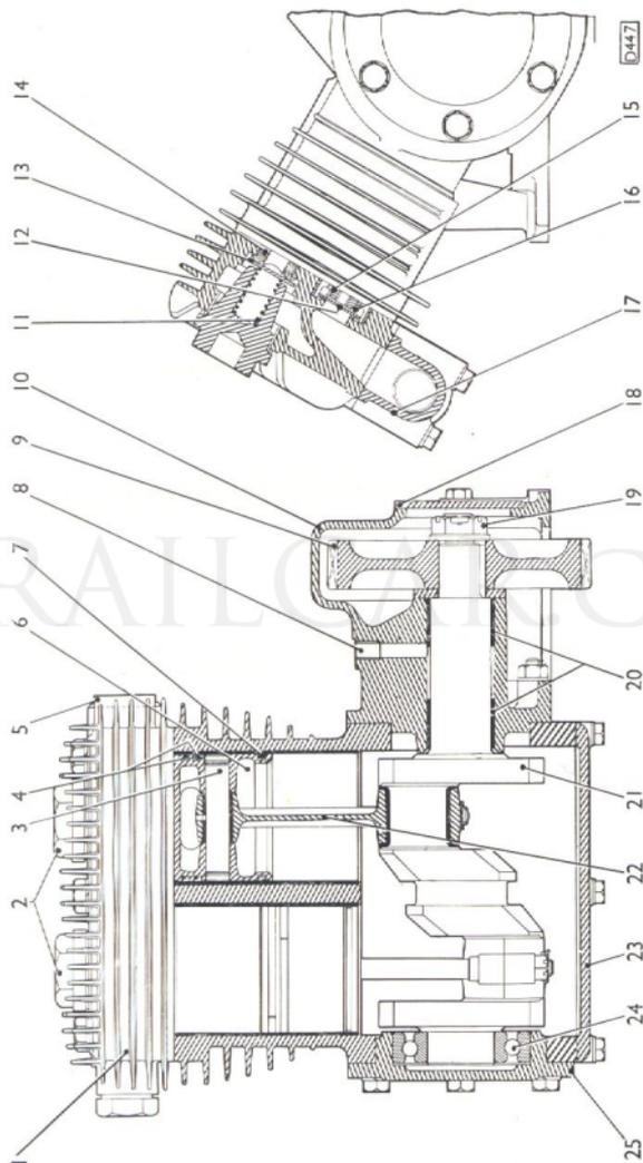
Fig. 71. Arrangement of air compressor.
