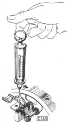
Fig. 70. Method of checking brush spring pressures.
