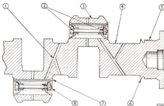
Fig. 17. Diagram of crankshaft oil passages.
