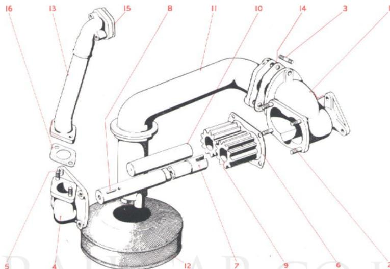
Fig. 16. Exploded view of the oil pump.
