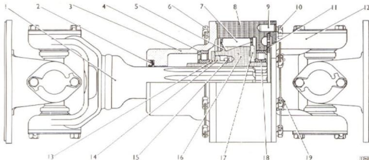
Fig. 3. Arrangement of first propeller shaft and freewheel.
