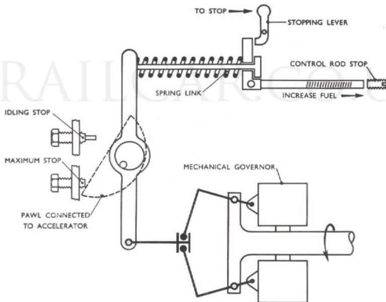
Fig. 80. Principle of the mechanical governor.
