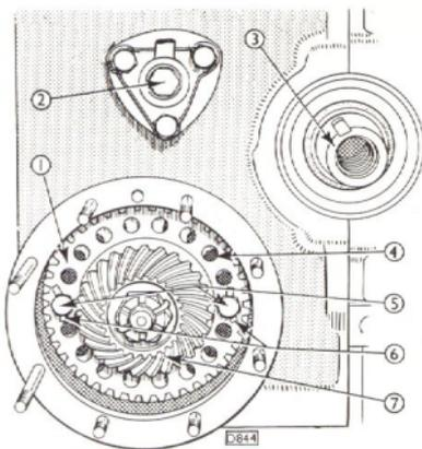
Fig. 14. Camshaft gear showing vernier adjustment.
