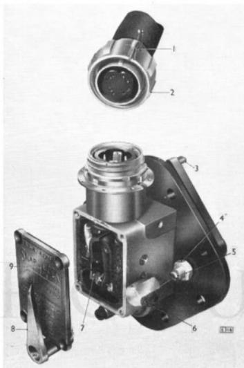
Fig. 38. Direction indicator switch.
