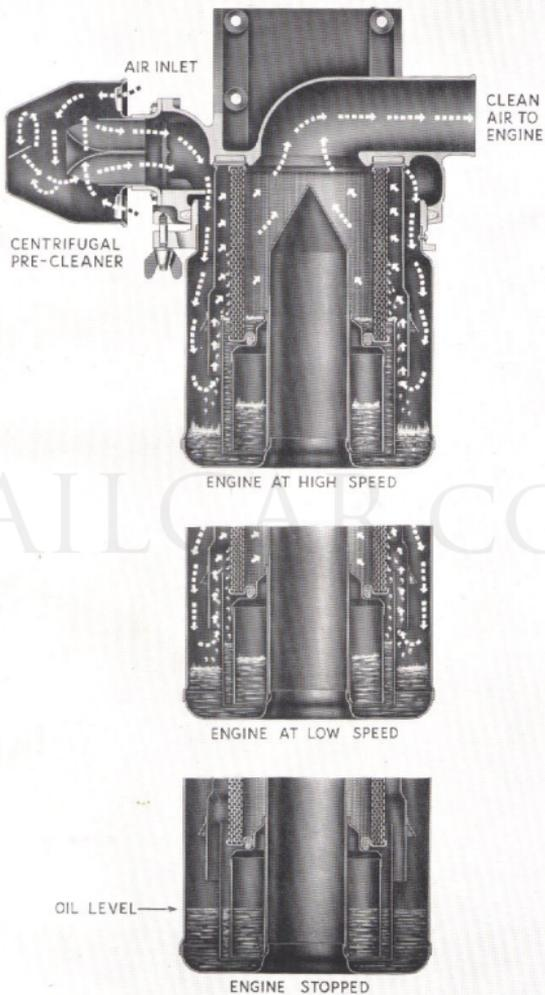
Fig. 93. Operation of the oil-bath air cleaner.
