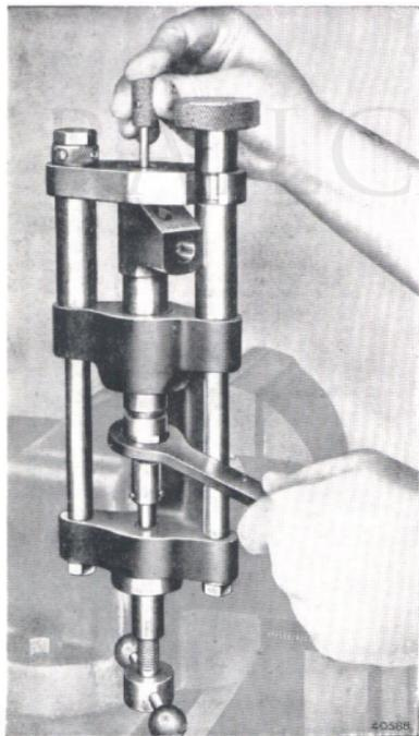
Fig. 71. Tightening the nozzle clamp nut.
