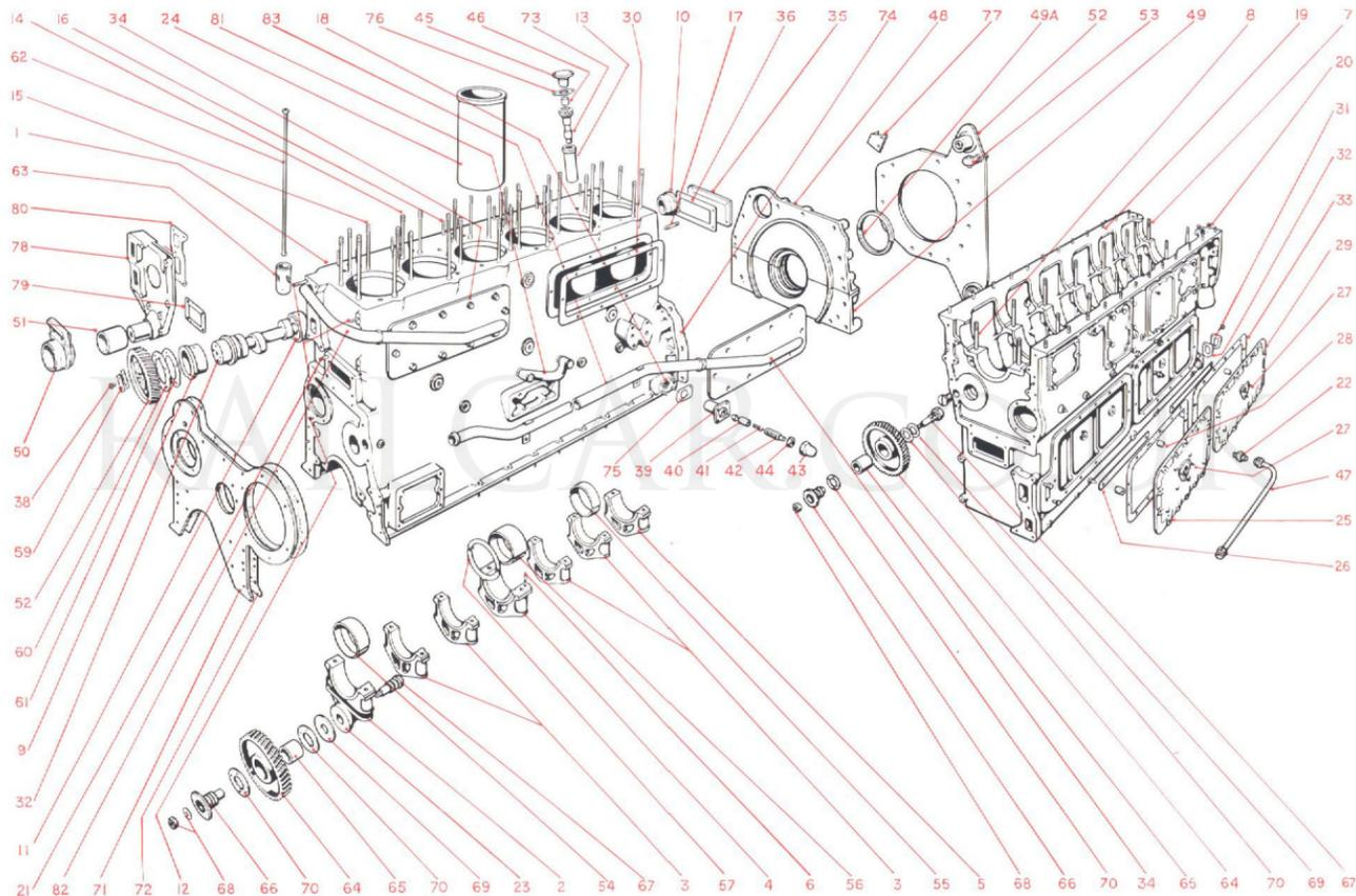
Fig. 17. Exploded view of the engine block.
