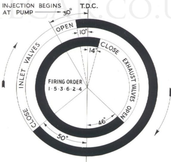
Fig. 6. Valve timing diagram.
