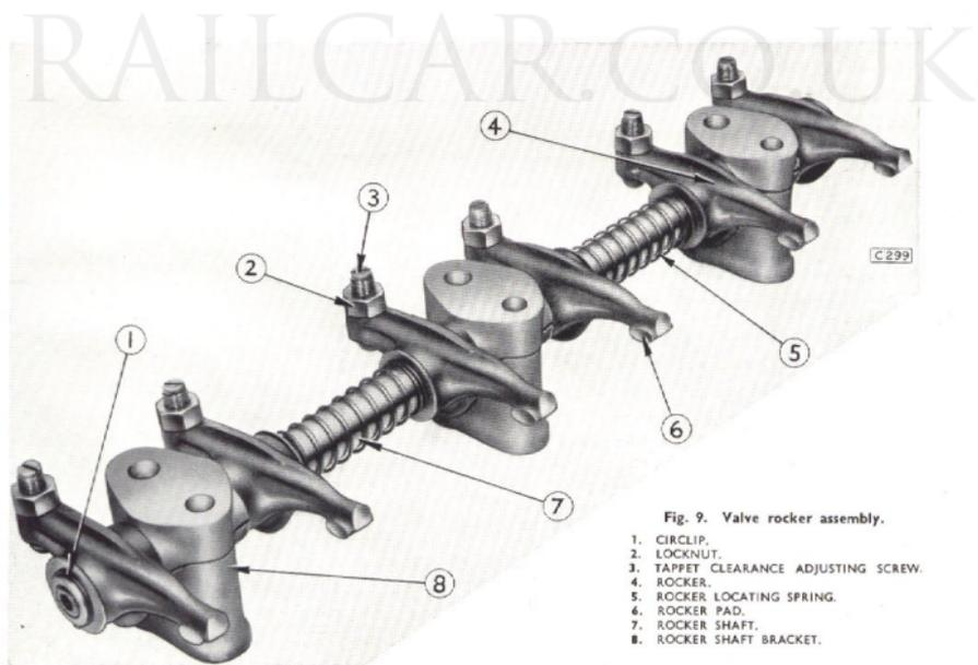
Fig. 9. Valve rocker assembly.
