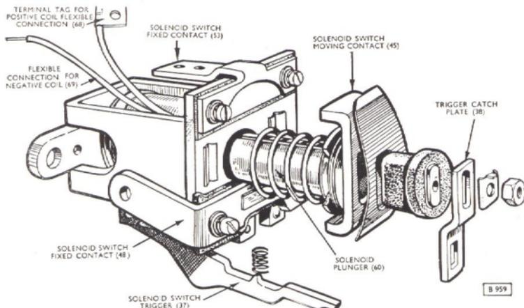
Fig. 66. Exploded view of starter motor solenoid switch (C.A.V.)
