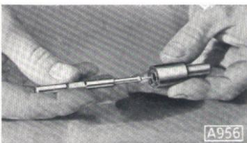
Fig. 28. Tool for cleaning nozzle tip.
