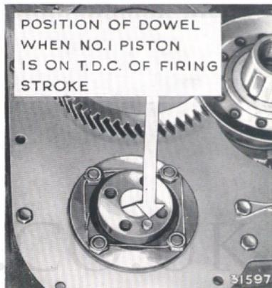
Fig. 39. Gear location in camshaft end.
