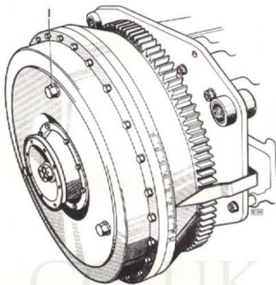
Fig. 13. Position of the flywheel for inlet valve opening.
