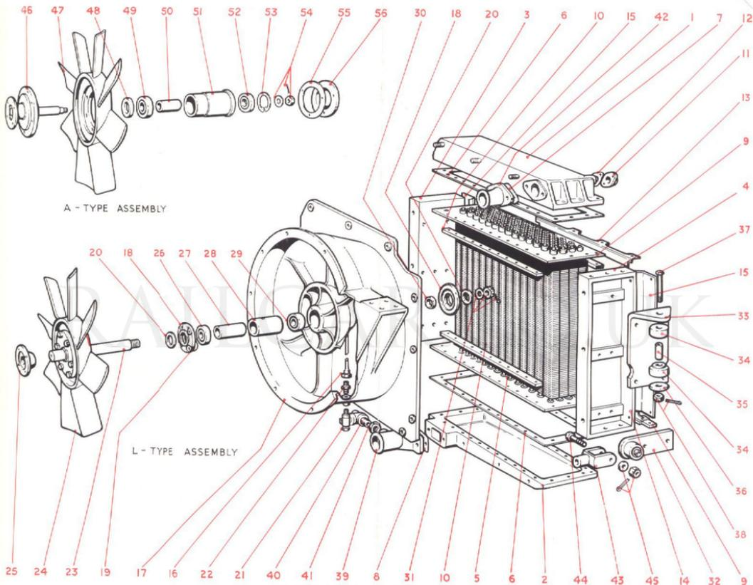
Fig. 3. Exploded view of radiator and fan.
