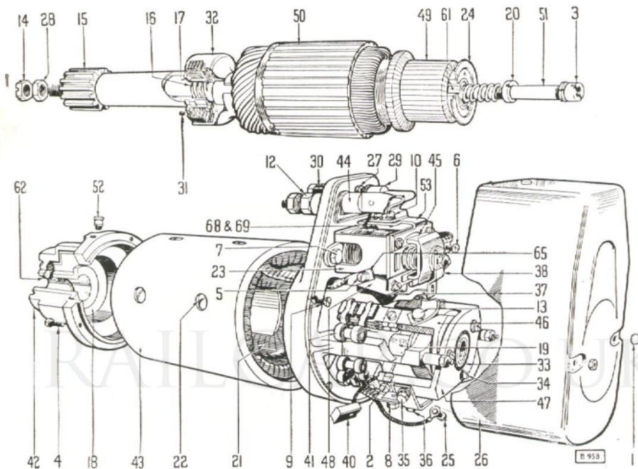
Fig. 63. Exploded view of C.A.V. starter motor.
