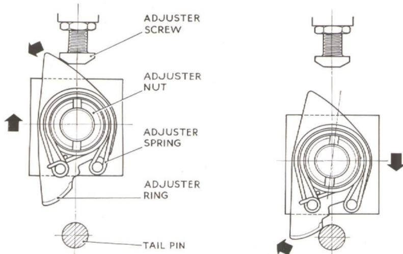
Fig. 5. Operation of the Automatic Adjuster.
