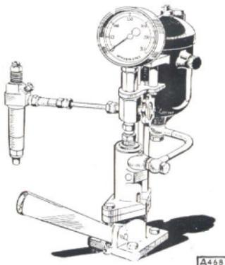
Fig. 25. C.A.V. hand-testing pump for injectors.
