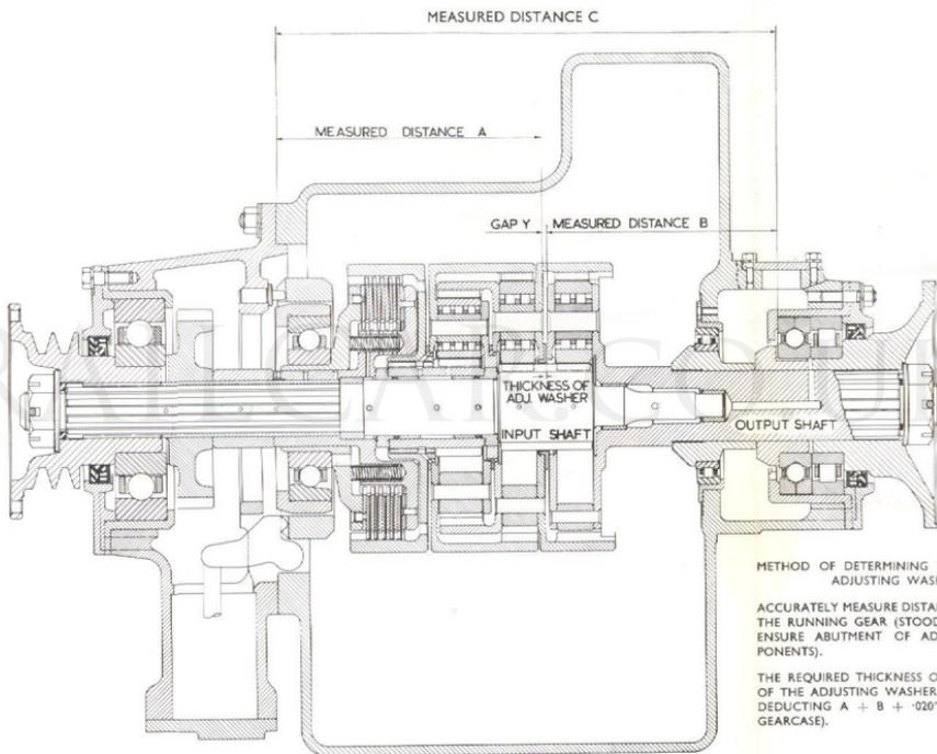
METHOD OF DETERMINING THICKNESS OF ADJUSTING WASHER
