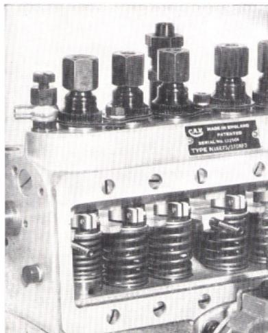
Fig. 78. The pump control quadrants.
