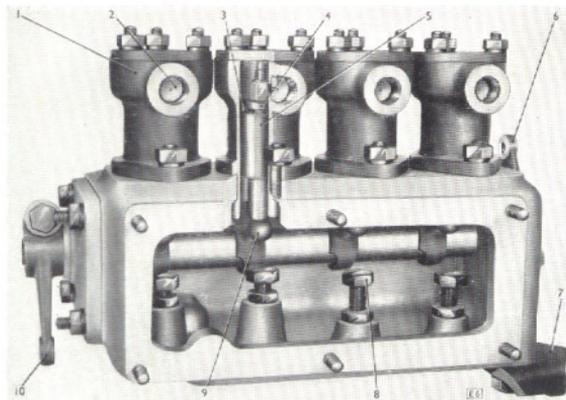
Fig. 10. Throttle motor showing adjusting screws.
