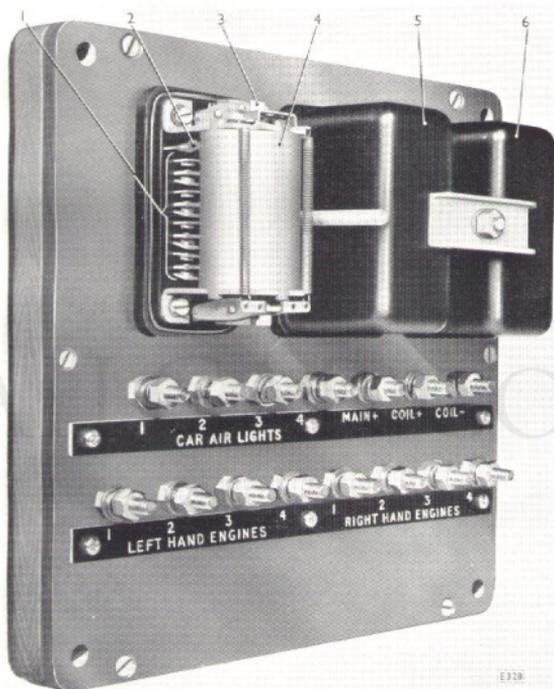
Fig. 20. Relay-operated switch panel (12 way).
