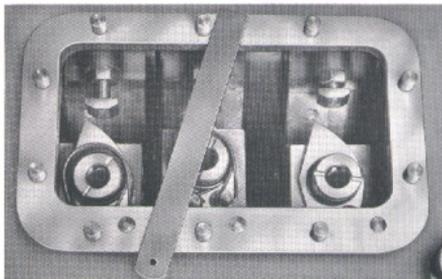
Fig. 15. Checking Movement of Adjuster Nut.
