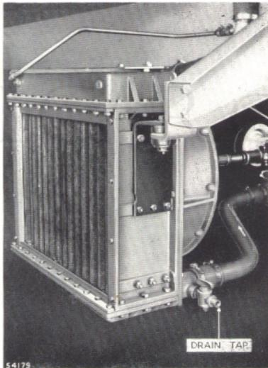
Fig. 1. Radiator showing position of drain tap.
