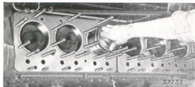
Fig. 41. Fitting the piston.
