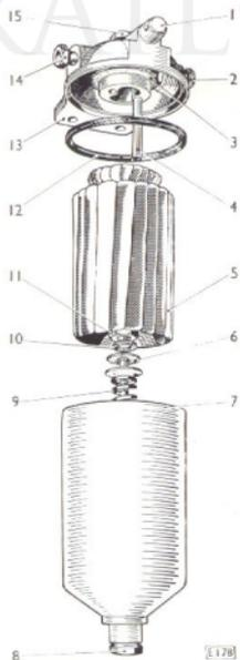
Fig. 45. Exploded view of main fuel filter (C.A.V. cloth element type).
