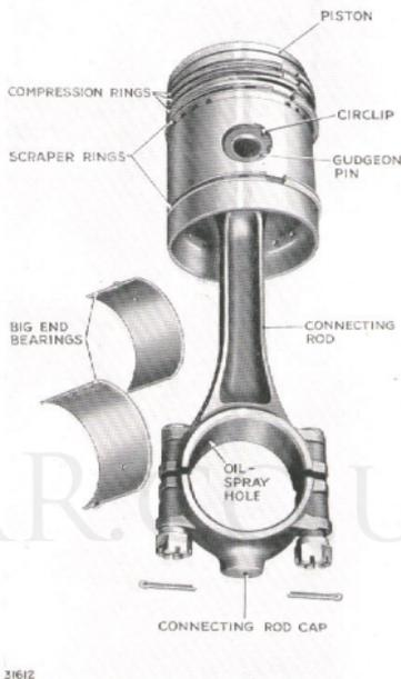
Fig. 42. Piston and connecting rod assembly.
