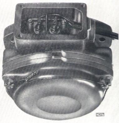
Fig. 72. Engine speed indicator generator—with cover removed.
